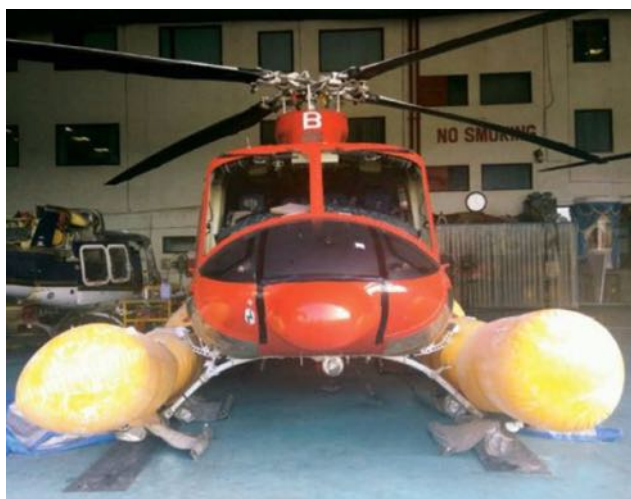
A civilian Bell 412 with flotation gear deployed.
