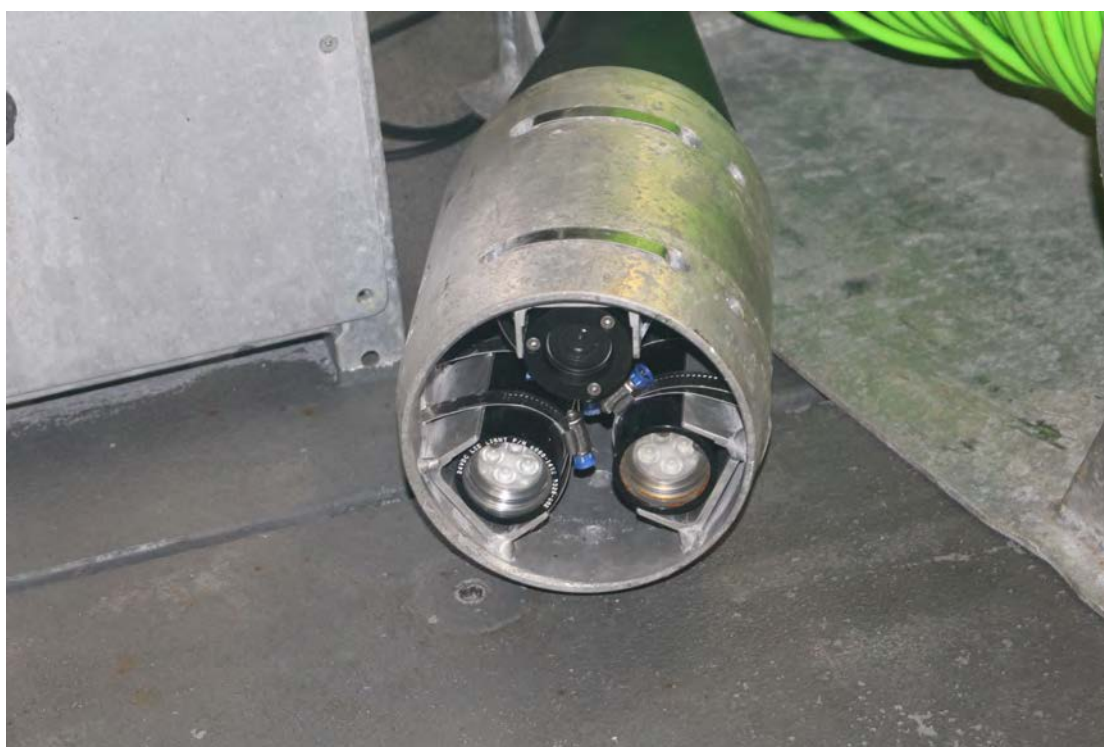
Figure 14 – Drop Camera showing two lights and lense
