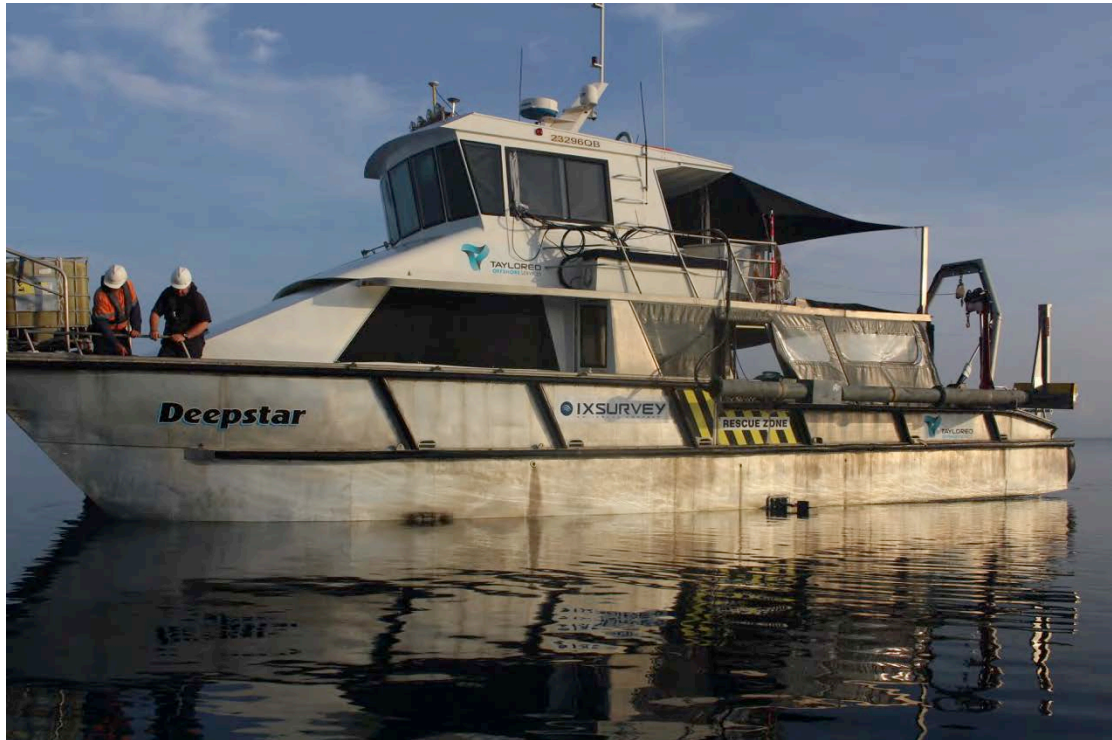
Figure 2 – Deepstar with MBES transducers on the right hand end of the raised pole
