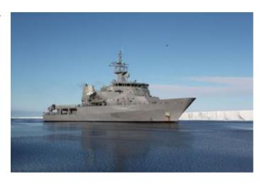
Zealand's 15,000 kilometer coast, the southern ocean and into the pacific. Both OPV's are designed to undertake patrols where ice may be encountered. They have a strengthened hull, but are not designed as
